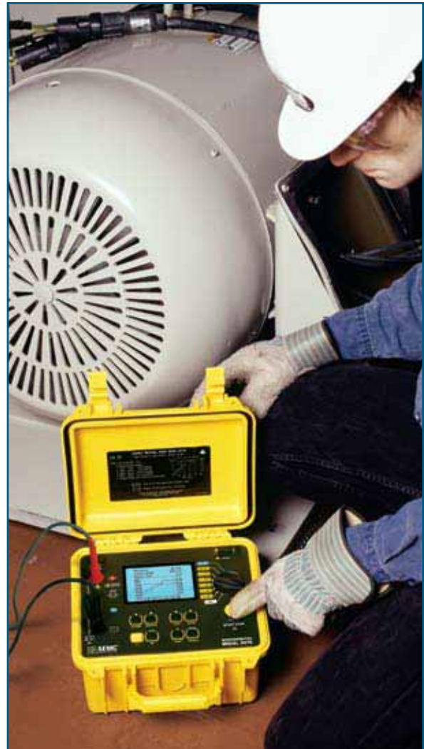
Model 5070 checking insulation resistance on feed cables to a three-phase motor.
