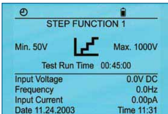
Step Voltage start screen shows start and ending test voltage, test run time and some of the parameters to be monitored
