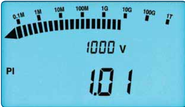
Automatic calculation and display of PI Ratio.
