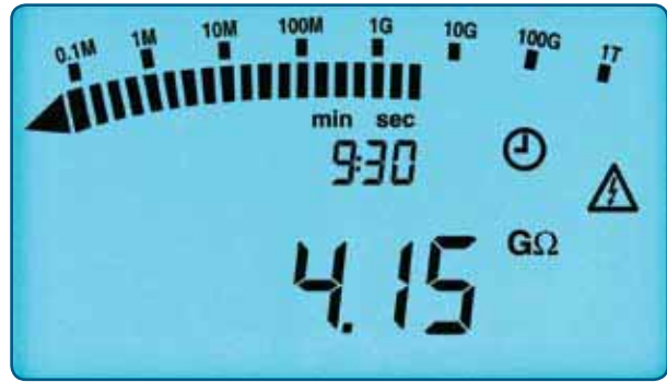
Automatic calculation and display of DAR ratio.
