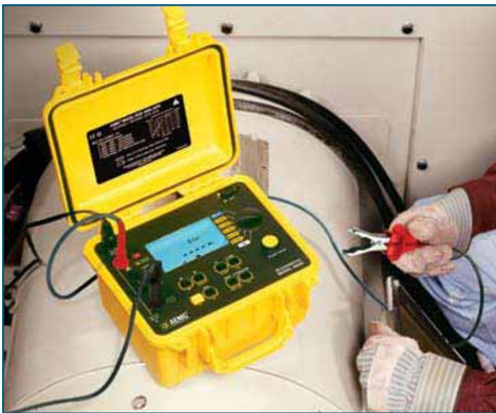
Model 5060 performing insulation test on a generator.
